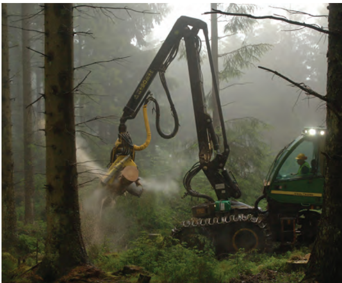
Figure 1 Falling trees and large machines are dangerous and can kill. They require a risk zone (typically of 50–70 m) from which the public must be excluded for their safety.
