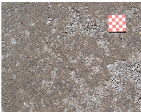
Foamed bitumen path with added cement.
